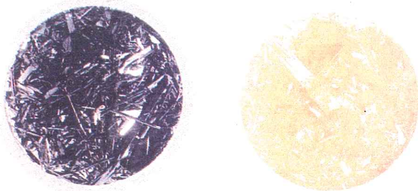
Fig.4 Cadmium sulphide has extension of prohibited Fermi's band of 2.6 eV and for this reason appears yellow, whereas cadmium selenide with a value of 1.7 eV is black. The reddish colours are intermediates. Adapted from F.Celentano "Luce colore e materia", Le Scienze, quaderno 21, Febbraio 1985.
